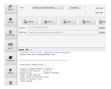
The screen should now look similar to the above. Press Program to re-program the PIC. When programming has finished, remove the PICkit3 from the CPU board and the calculator should be functioning as a HP-31E. Turn the calculator OFF and refit the rear case half.
