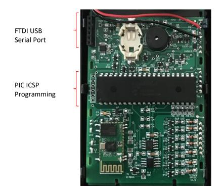
Note: All connection to the PC RS-232 or PIC programmer should be connected or disconnected while the calculator is turned ON.
