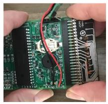
Try pushing in one end a bit, then the other end and continue until the bottom edge of the display is parallel and about 1mm from the top edge of the CPU board.
