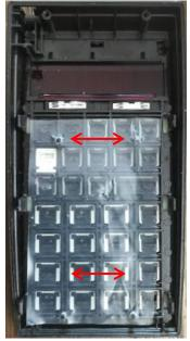
If desired, and originally fitted, the retaining clips can be clipped onto the new boards.
