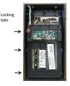
The CPU assembly locking tabs need to be bend outward at the three positions shown. This can be a bit difficult but you should be able to pull one tab and raise the CPU board a bit, then move on to the next tab.
