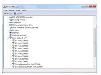
Run CalCom.exe and you will get a connection error message if the operating COM Port number does not match the one assigned to the Bluetooth module.
