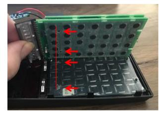
Position the CPU board as shown and make sure the far edge of the board is underneath the 3 locking tabs as far as practicable. Line up the two holes in the CPU board with the two posts in the top casing.
